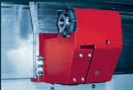
**Tailstock.** On the MAXXTURN 45 with tailstock, the tailstock is set up on the linear roller slide and can be automatically positioned within a range of 510 mm. The live center is integrated into the body of the tailstock and can be removed using a pressure wedge.
