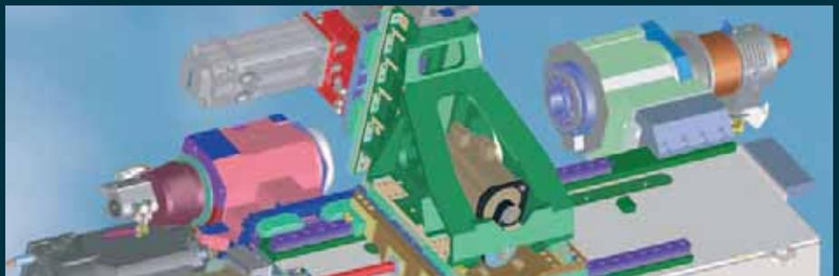
**Y axis.** The Y axis is integrated into the basic machine structure and stands at 90° to the X axis. Extremely short projections form the basis for solid turning and drilling operations, as well as milling operations without interference contours.
