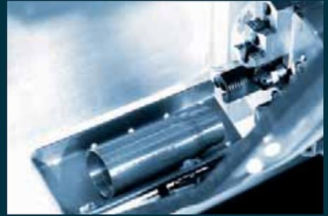
**Counter spindle and parts catcher.** The counter spindle includes a parts ejector with stroke monitoring and coolant feed. It ejects the parts automatically into the parts catcher, which then removes them from the machine and stores them in a bin or on an accumulating conveyor.
