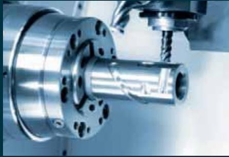
**Main spindle.** The main spindle with large precision bearings allows a very wide range of speeds, combined with extremely good true running characteristics. Cooling fins are fitted to the symmetrical headstock to ensure optimum thermal stability.
